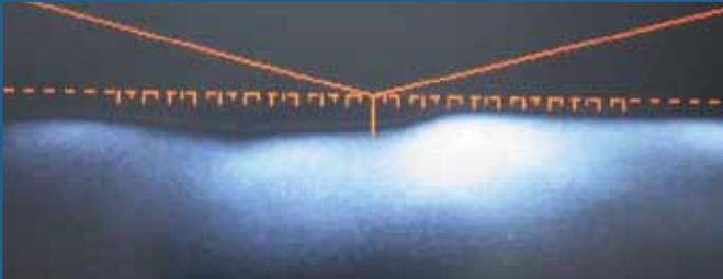
Filtered live image of a Bi-Xenon headlight on the HTD 815 headlight tester with a clear cut-off line
