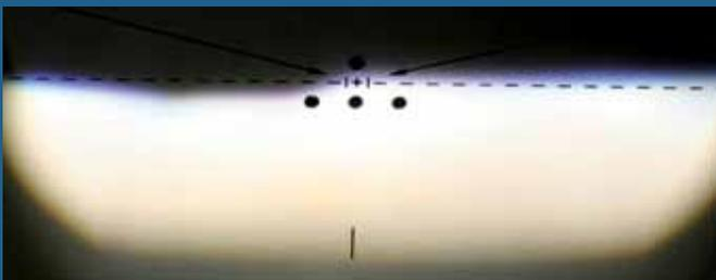
Bi-Xenon headlight image on an analog headlight tester
